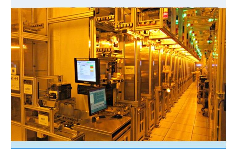
In SSMC Annex10 Cleanroom, AMHS (Automated Material Handling System) and Autoloaders are deployed to enable lots to travel autonomously from machine to machine, bay to bay across the cleanrooms. This highly automated operation is one of the key ingredients of SSMC's productivity strategy, towards manufacturing excellence and total quality.
